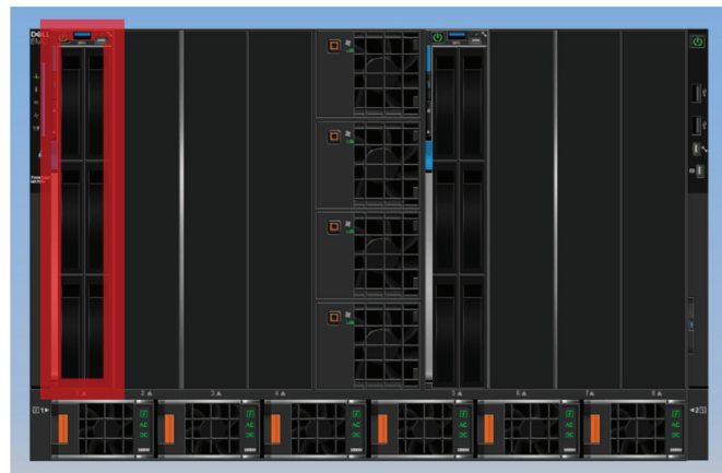
Figure 7. NOM-A1-01-10a and NOM-A1-01-10b are blade servers inside NOM-A1-01-10
